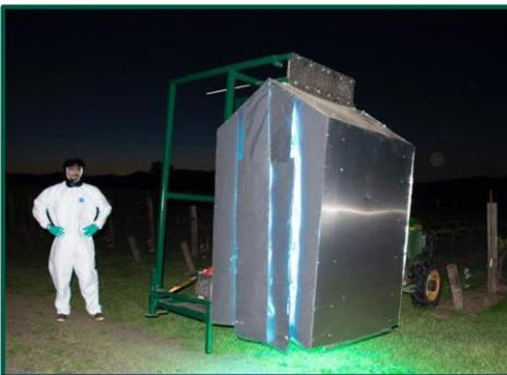
Tractor mounted UV-C array in operation at night
